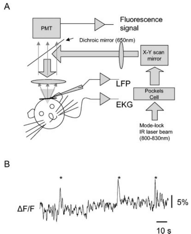
Fig. 3. Two-photon imaging of fluorescence-labeled pericytes in vivo. **A:** Sketch of the imaging setup. The mouse is fixed with a metallic head frame and mounted rigidly under a custom-built two-photon laser-scanning microscope. **B:** An example trace of Calcium Green fluorescence imaging in a pericyte. Sporadic  $\text{Ca}^{2+}$  surges are marked by asterisks.
